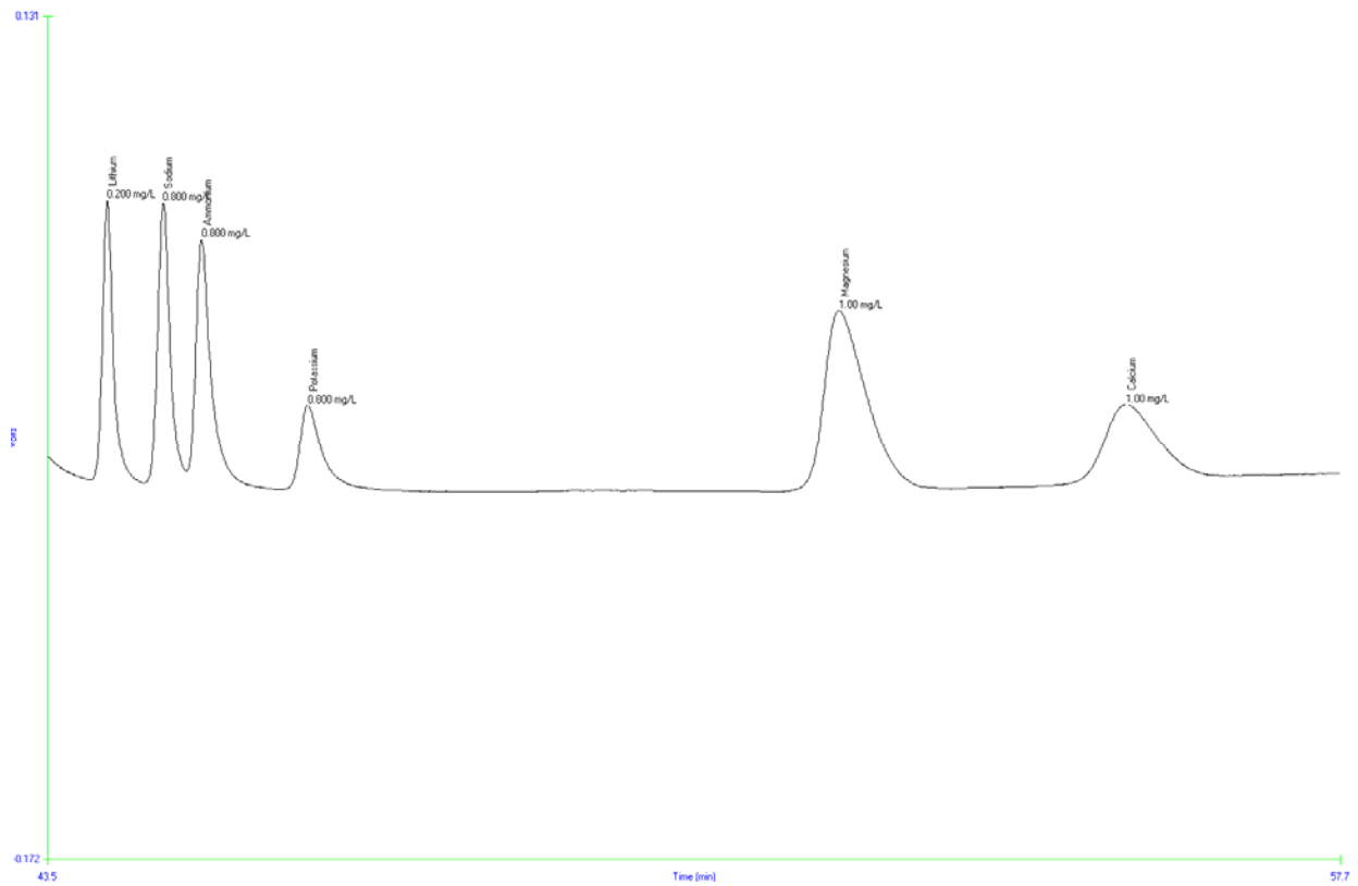
Chromatogram showing separation of Standard C using the PN 2809 cation profiling column. Range 2. Date acquired: 25 Oct 2004
